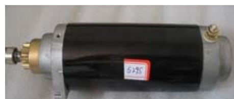
5295 MERCURY MARINE:50-55304A1 12V 10T CCW
